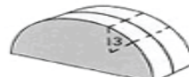
Cut out notch about 1/3 of the way up one end of body.
